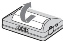
**2** Insert a size-AA alkaline dry battery (minus terminal first).
