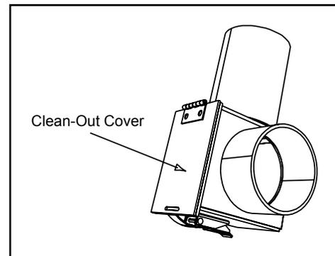
**Figure 18.3 - Rear to Top Vent Adapter - 90°**
