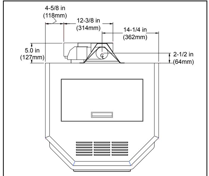
**Figure 7.2 - Top View with Top Vent Adapter**
