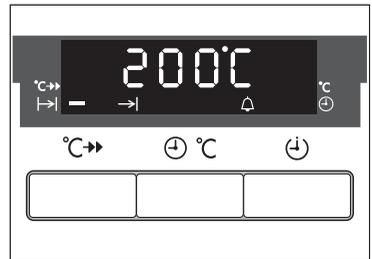
When the time has elapsed, "0.00" and the function indicator flash.
