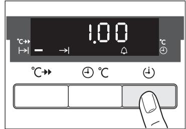
3. Using the End time →| function, set the time at which the dish should be ready.
