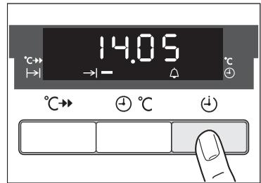
The Cook time |→ and End time →| function indicators light up and the temperature is shown in the display.
