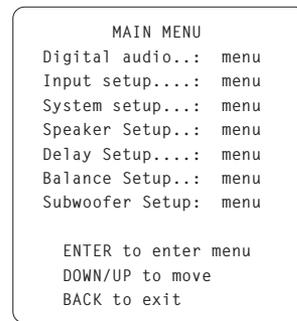
The MAIN MENU screen is the entry point for all of the RSP-985's settings and setup menus where system configuration settings can be made. These are typically accessed only during initial system configuration and are not used in day-to-day operation:
