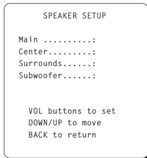
This menu, which is reached from the MAIN menu, allows you to configure the RSP-985 to make optimum use of the capabilities of the speakers in your system. Using these settings, the RSP-985 adjusts its crossovers and digital processing to direct signals to the appropriate speakers.
