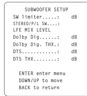
This menu, also reached from the MAIN screen, allows you to optimize the RSP-985 for your particular subwoofer. The settings in this menu may be considered to be “advanced” and need not be adjusted unless specifically desired.
