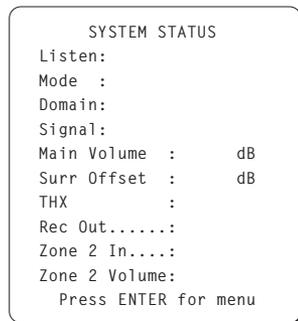
The SYSTEM STATUS screen provides the status all of the important settings of the RSP-985 and a starting point for reaching all other screens and menus. This screen is available at any time by pressing the ON-SCREEN button on the remote control. The screen displays the following status information:
