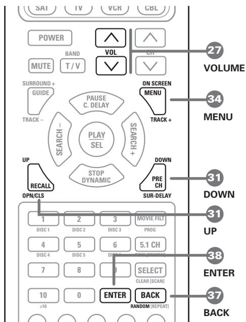
The following buttons are used to navigate the ON-SCREEN MENU system:
