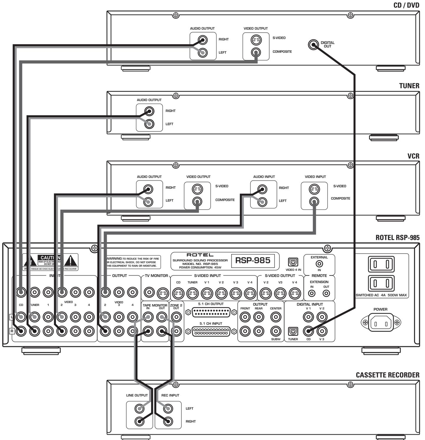
Figure 5 – S-Video Source Connections
