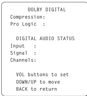
This menu, which is reached from the MAIN MENU, provides status information and setup options for digital inputs.
