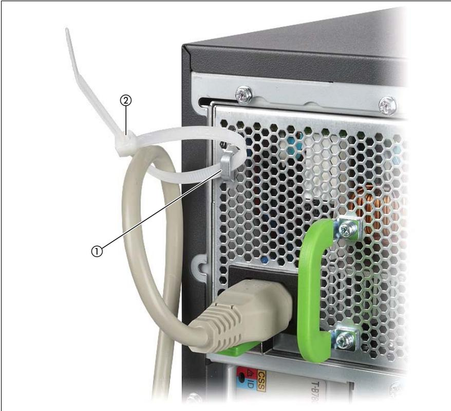
Figure 11: Using cable ties
