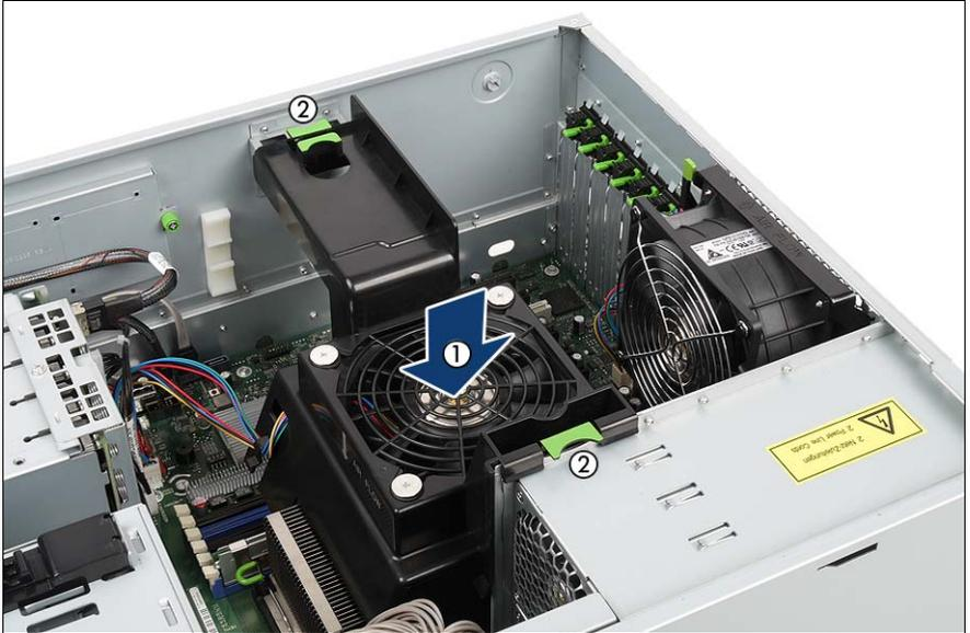
Figure 37: Installing system fan 2 (and 4)
