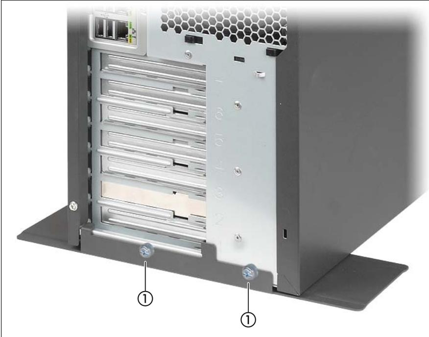
Figure 2: Mounting the anti-tilt bracket
