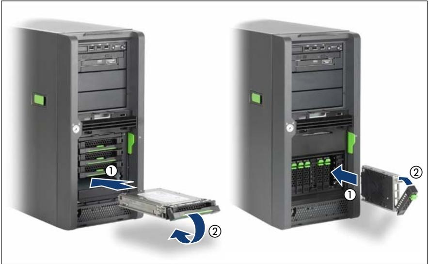
Figure 26: Installing the 3.5-inch and 2.5-inch HDD modules
