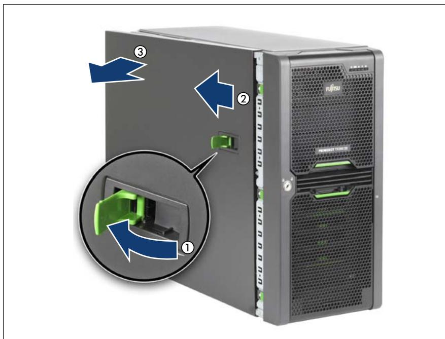
Figure 27: Opening the server (example: floorstand model)
