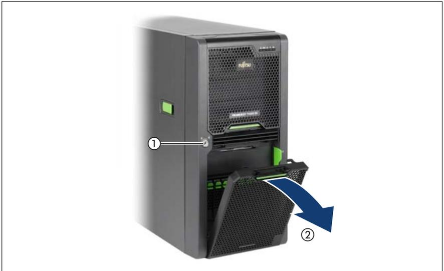
Figure 14: Removing the hard disk cover
