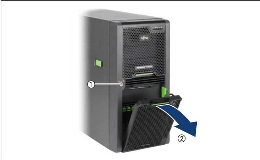
Figure 23: Removing the hard disk cover
