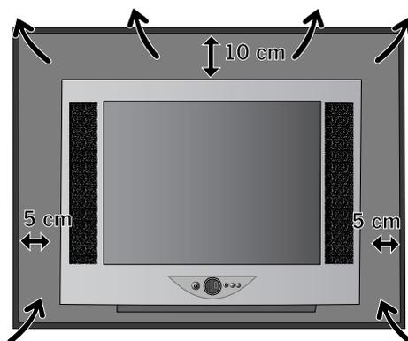
If the TV set is placed in a cabinet or on a shelf, at least 5 cm clearance at the sides and at least 10 cm at the top must be left to allow air to circulate. Stand the TV set in a place where it is not exposed to direct sunlight or additional heating from radiators.
