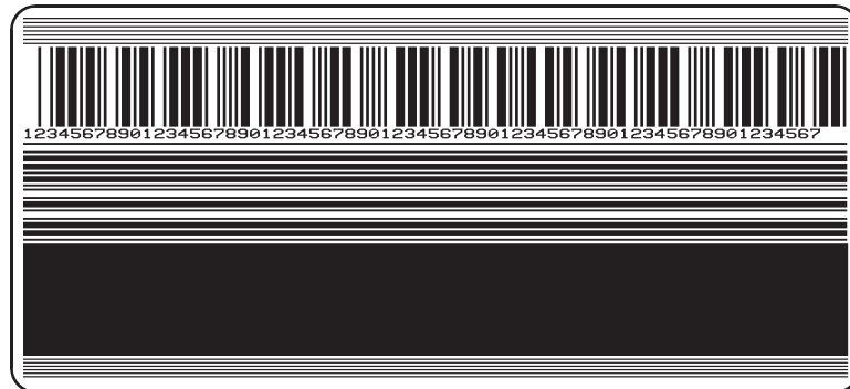
Figure 17. Pause Key Test Sample Printout
