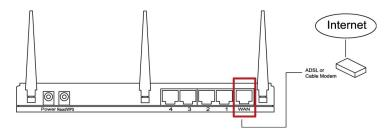
Standard modems provided by Internet Service Providers (also referred to as ISPs) come with at least one LAN or Ethernet port. This is the port which you need to connect to the WAN port of the INTELLINET NETWORK SOLUTIONS Wireless N Gigabit Router.
