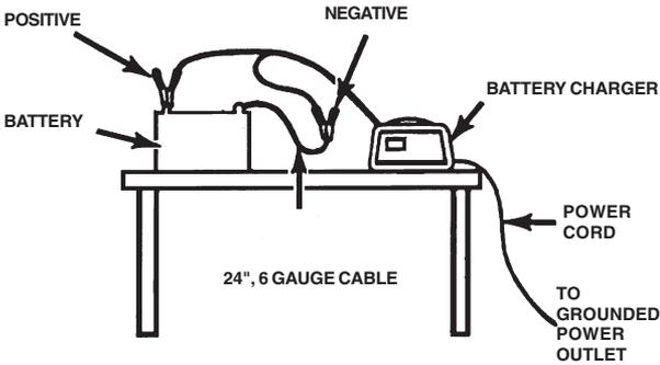
1. Note the polarity of the battery posts by checking the identification marks on the battery: POSITIVE (POS, P or +) and NEGATIVE (NEG, N or -). The positive post is usually larger than the negative post.
