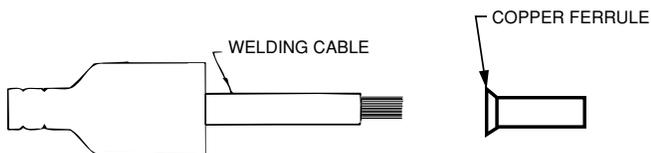
5. Slide the copper ferrule into the brass plug.
