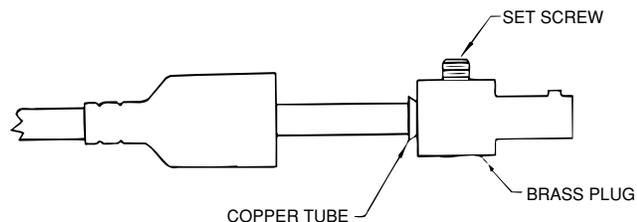
7. Slide rubber boot over brass plug. The rubber boot must be positioned to completely cover all electrical surfaces after the plug is locked into the receptacle.
