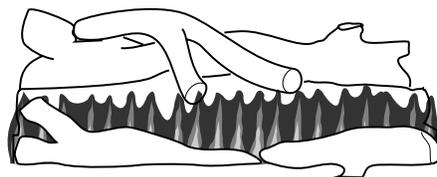
Figure 27 - Correct Front Burner Flame Pattern
