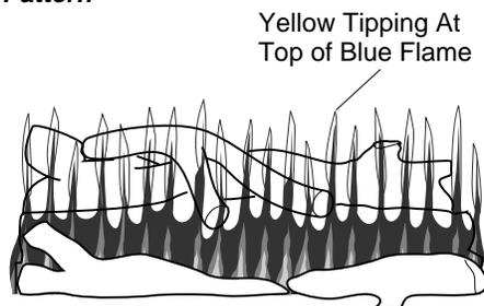
Figure 28 - Incorrect Front Burner Flame Pattern
