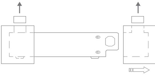
Open the box from the top and remove the accessories from the foam end caps. You may now proceed to lift the unit from the box. Once the unit is removed you can proceed with the removal of the foam end caps. These caps are designed to fit on the front and back of the unit for maximum protection. Retain the packaging for future transportation of this unit.
