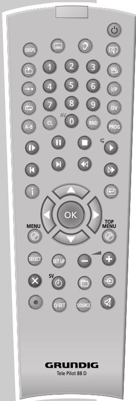
**SELECT** Switches between external USB source and HDD archive.
