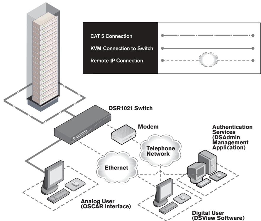
Figure 2.1: The DSR1021 Switch in a Network Configuration
