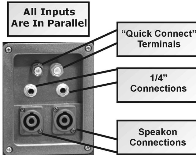
Make certain that the wires you are using are at least 12 gauge unshielded speaker cable (the lower the number, the thicker the wire). Do not use shielded "instrument" cables.
