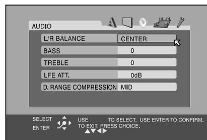
There are five items on the Audio Menu to tailor the audio performance of the system. These adjustments can also be made from the front panel and/or remote control as described in the Comprehensive Setup and Sound Settings sections of the manual.
