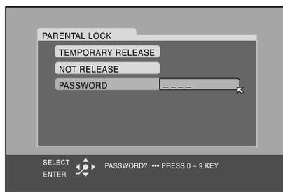
1. To eject the disc, use the CURSOR ▲/▼ buttons on Page 1 of the remote to highlight the NOT RELEASE field, then press the OK button. Eject the disc.
