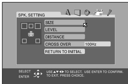
There are four items on the Speaker Setup Menu to configure the RSDX-02 for proper operation with your system. These adjustments can also be made from the front panel and/or remote control as described in the Sound Settings section of the manual.
