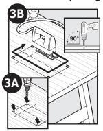
**3A** Drill ½" holes in inside corners of drawn template. These will be the pilot holes for the saw blade.
