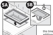
**5A** Place interior frame (frame with 2 flaps) into cut-out. Next place exterior frame into cut-out from under side of door, inserting core covers inside tabs of frame. Hold frame together. Insert nylon screws through holes in interior frame into holes in exterior frame. Thread a hex nut onto bottom of each screw.
