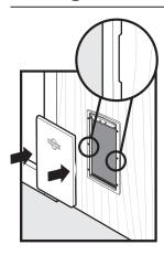
The Closing Panel snaps onto the interior frame of the Extreme Weather Pet Door $^{\text{TM}}$ . It is useful during inclement weather or to keep your pet from using the pet door.
