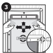
Replace flap clamp with attached insulated flap. Insert new vinyl flap between flap clamp and flap screw holes in top of frame. The PetSafe® logo should be readable on vinyl flap, Replace flap support, Alian screw holes in flap support, frame, vinyl flap and flap clamp. Replace and start screws to hold flap in place. Adjust flap horizontally until centered in pet door frame. Adjust flap vertically until magnet bar on frame jumps to meet magnet on bottom of flap. Tighten screws.
