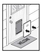
An additional closing panel (sold separately) can be used on the exterior frame of the Extreme Weather Pet  $\mathsf{Door}^\mathsf{TM}$  for improved weather resistance. See "Replacement Parts and Accessories" on page 10.
