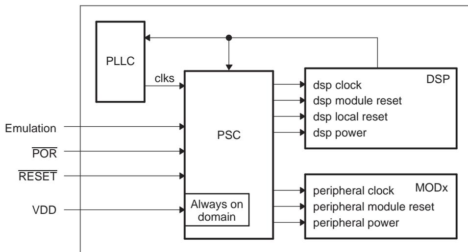
NOTE: The effects of DSP local reset and DSP module reset have not been fully validated; therefore, these resets are not supported and should not be used. Instead, the  $\overline{\text{POR}}$  or  $\overline{\text{RESET}}$  pins should be used to reset the entire DSP.
