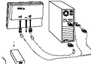
5. Plug the AC power cord into the FPD. Alternately, you can use the optional power supply from 3M.
