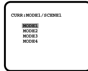
4. The camera is now in scene file set mode and as shown on the right figure on the top appear on the monitor screen.
