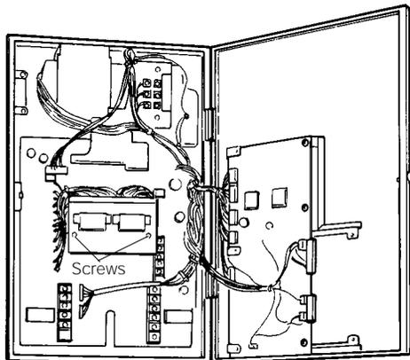
(2) Fit the two spacers on the connector board and fasten the circuit board with the screws removed in Step (1).
