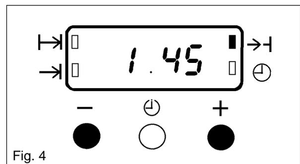
The 'Countdown' will sound intermittently for up to 2 minutes at the end of the timed period. The sound can be stopped by pressing any button.
