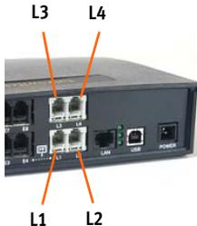
For TalkSwitch 48-CA and 48-CVA, connect a **four-wire** RJ-11 telephone cable to the wall phone jack of the incoming phone lines and the other end to the L1/L2 jack of the TalkSwitch unit.
