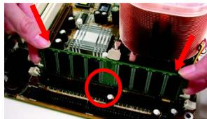
1. Unfasten the clips on each end of the memory slots. Correctly align the memory module in the slot and push downwards..
