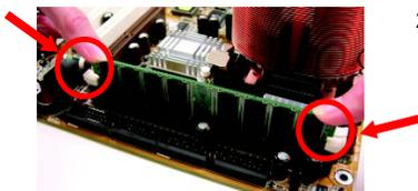
2. Once the memory module is correctly inserted, the clips will automatically refasten. If the memory module is positioned in the wrong direction, it will not insert. If this occurs, please switch directions.
