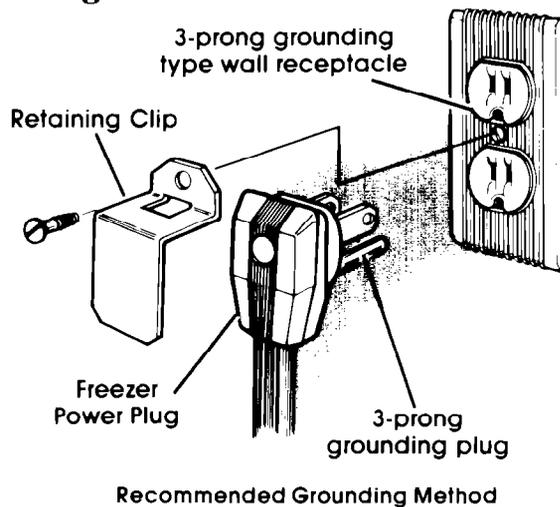
A 115 Volt, 60 Hz., AC only 15 or 20 ampere fused and properly grounded electrical supply is required. It is recommended that a separate circuit serving only this appliance be provided.
