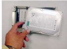
4. Connect the hard disk connector into the inner tray's slot.
