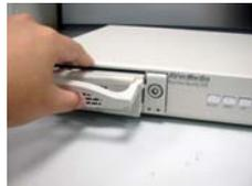
6. Power on the unit to see the LED indicators on the triple frame holders. If the LED indicators light up, you may use the hard disk.
