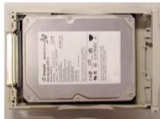
5. Close the upper cover. Slide the drawer into the removable hard drive case.
