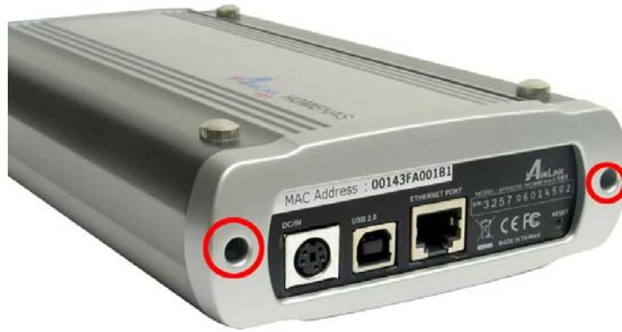
**Step 2** Pull out the front panel.
