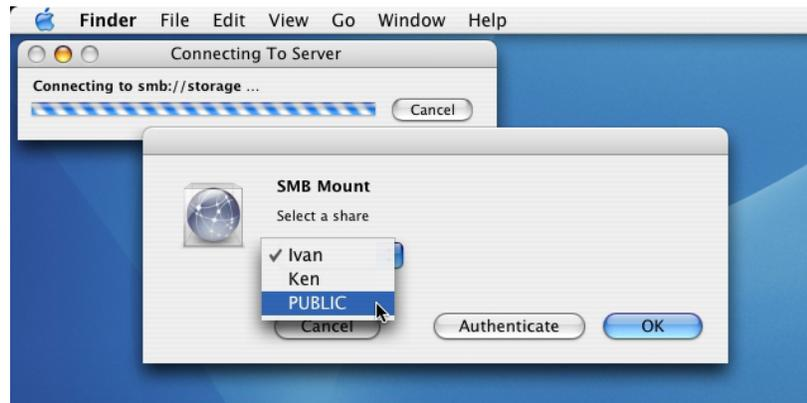
You might be prompted to enter a password, unless a password was previously assigned in the control panel, you can leave it blank. After a successful mount, a network folder icon will be created based on the folder you selected as shown.
