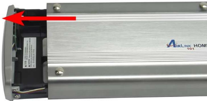
**Step 3** Put the 3.5-inch IDE hard disk into the plate, and connect the IDE and power cables to your hard drive.
