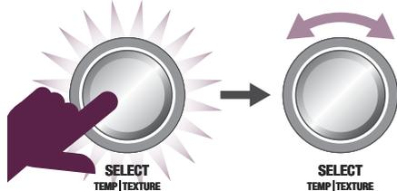
Press SELECT dial to set and the current polishing time will flash. Turn SELECT dial to select 2-7 seconds. Press SELECT dial to set. Machine will beep once to confirm settings.
