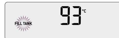
Fill tank with cold fresh water. The machine will not be able to make coffee or hot water while the tank is empty.
