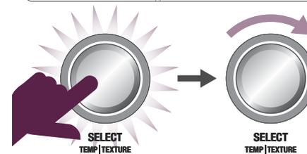
Turn the SELECT dial to the left or right to select the desired Auto Start time. Turning the SELECT dial faster or slower will change the rate of adjustment. When required time has been reached, press the SELECT dial to set. A small clock icon will be displayed on the LCD when the Auto Start function has been programmed.
