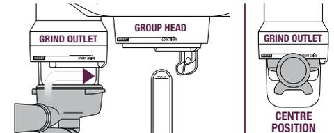
To start the auto grind, dose & tamp function, rotate the portafilter to the right then gently guide back to the centre position. Grinding will commence.
