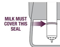
To start, press down and release steam lever. The LCD will display the temperature of the milk as it heats. Milk texturing will stop automatically when the selected milk temperature is reached. Lift steam wand to remove milk jug. **Wipe the wand & tip with a damp cloth.** Lower steam wand to the down position and the wand will automatically purge.
