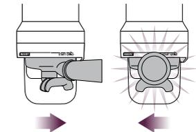
When the auto grind, dose & tamp function is complete, rotate the portafilter handle to the INSERT position and lower to remove.
