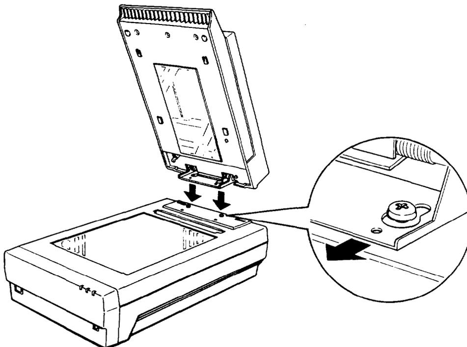
4. Use a coin to tighten the two screws and secure the transparency unit.
