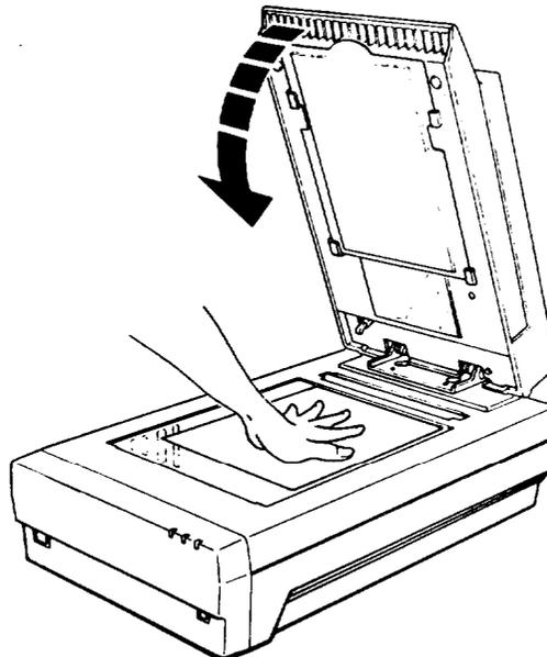
To remove the reflective document mat, lift up on the mat and pull it out of the transparency unit.
