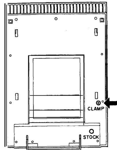
3. Insert the screw you just removed into the storage-hole in the position shown.
