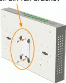
2. Mount the units on a din-rail chassis
