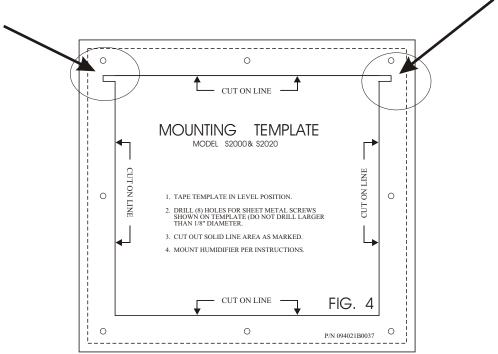
With this modification done, you should be able to insert the new humidifier into the cutout opening and secure the unit with the 8 self tapping screws provided. The hole dimensions on the front plate have not changed and should match up. If necessary, locally reinforce the opening with sheet metal sleeves to insure that the unit will remain level and not sag with the added weight of the water.
