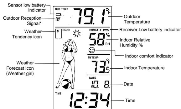
\*When the outdoor signal is successfully received by the Weather Station, this icon will be switched on. (If not successful, the icon will not be shown in LCD) So user can easily see whether the last reception was successful (icon on) or not (icon off). On the other hand, the short blinking of the icon shows that a reception is currently taking place.
