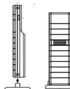
The Sensor is supplied with a holder that may be attached to a wall with the two screws supplied. The Sensor can also be position on a flat surface by securing the stand to the bottom to the Sensor.
