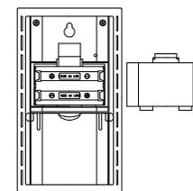
1. Remove the cover at the back of the Weather station.
