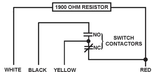
**THERMAL BALANCER SCHEMATIC DIAGRAM
