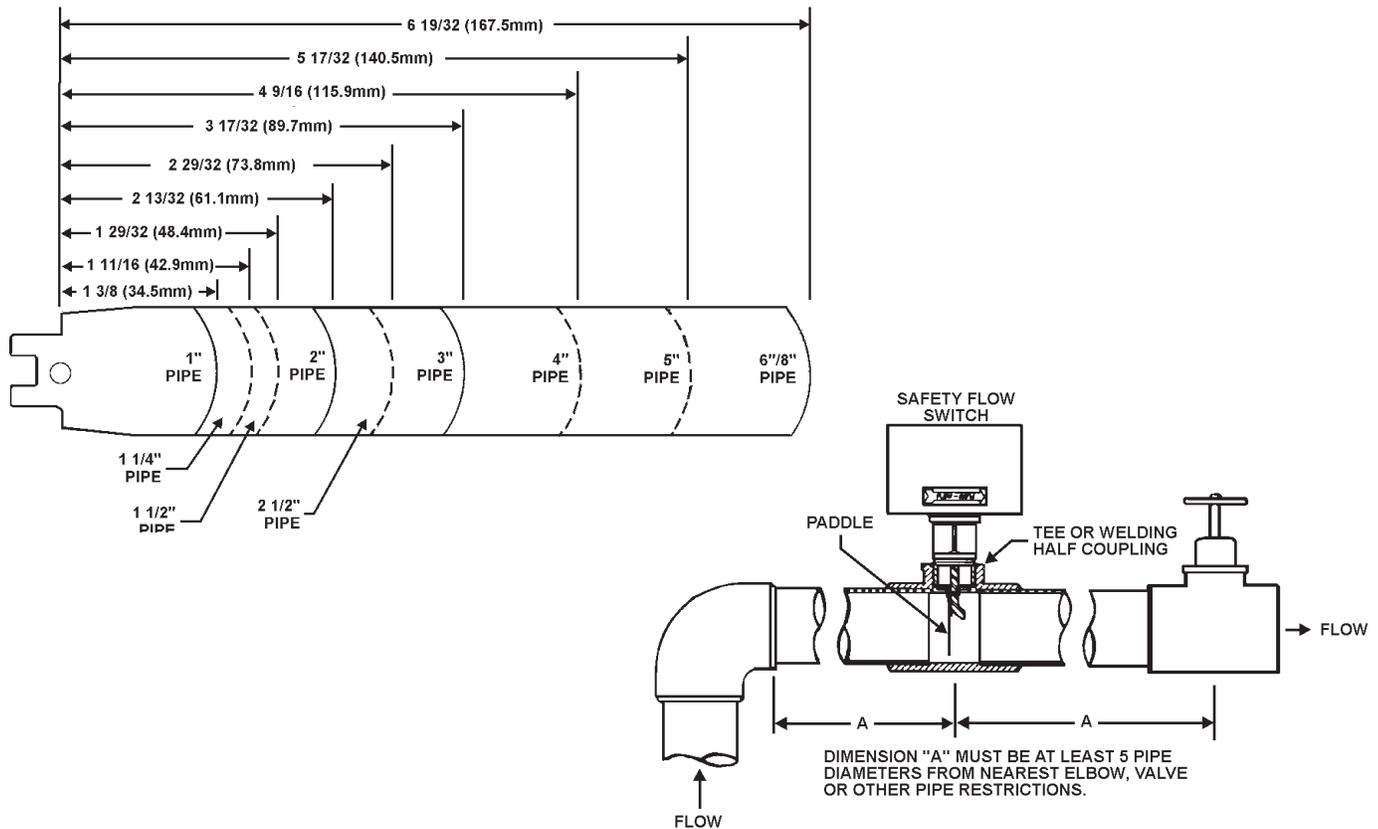
**CAUTION:** The paddle must be trimmed at the dotted arc. It must not touch the pipe or any restrictions when installed.
