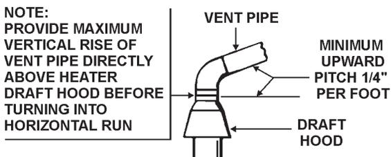
**PROPER VENT PIPE INSTALLATION
