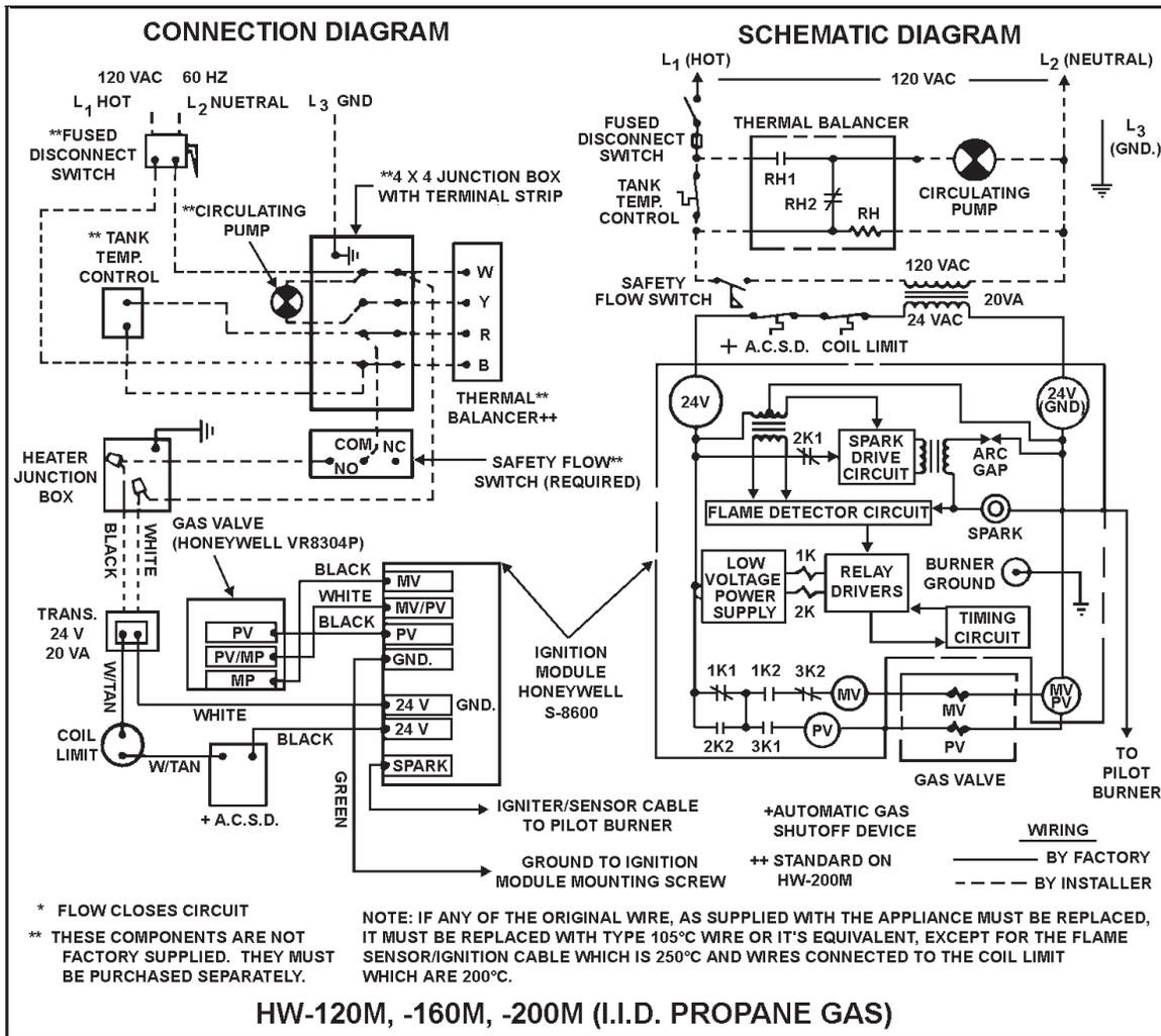
ELECTRICAL WIRING DIAGRAMS FOR THE HW-120M, 160M, AND 200M WATER HEATERS
