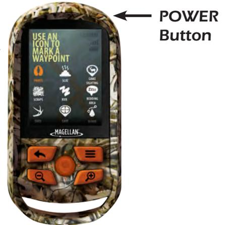
**Hard Reset:** In the unlikely event that the device becomes "locked up" or is behaving erratically, you can perform a hard reset which will probably cure the problem. Open the USB cover and locate the small hole that provides access to the reset button. Insert a paper clip or other small object in the hole and quickly press the reset button. The device will turn off and then turn back on. Note: If planning a trip you will lose all information for that trip.
