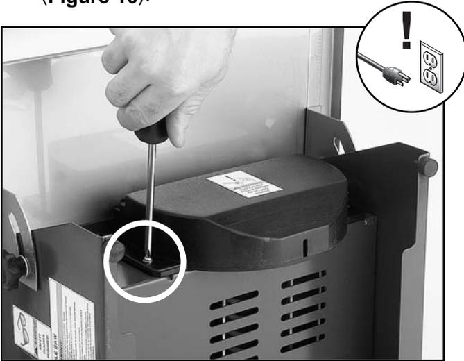
Figure 10. Loosening one of the blade cover screws.
