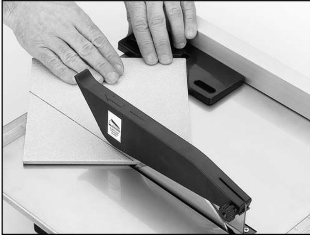
**Figure 8.** Diagonal cutting with the miter gauge.
