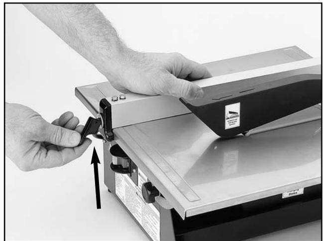
**Figure 7.** Rip fence locking lever.
