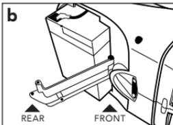
from the bracket. If the battery has leaked or vented, protective gloves should be worn before touching the case. Remove the case by grasping the edges and sliding the battery out of the unit.
