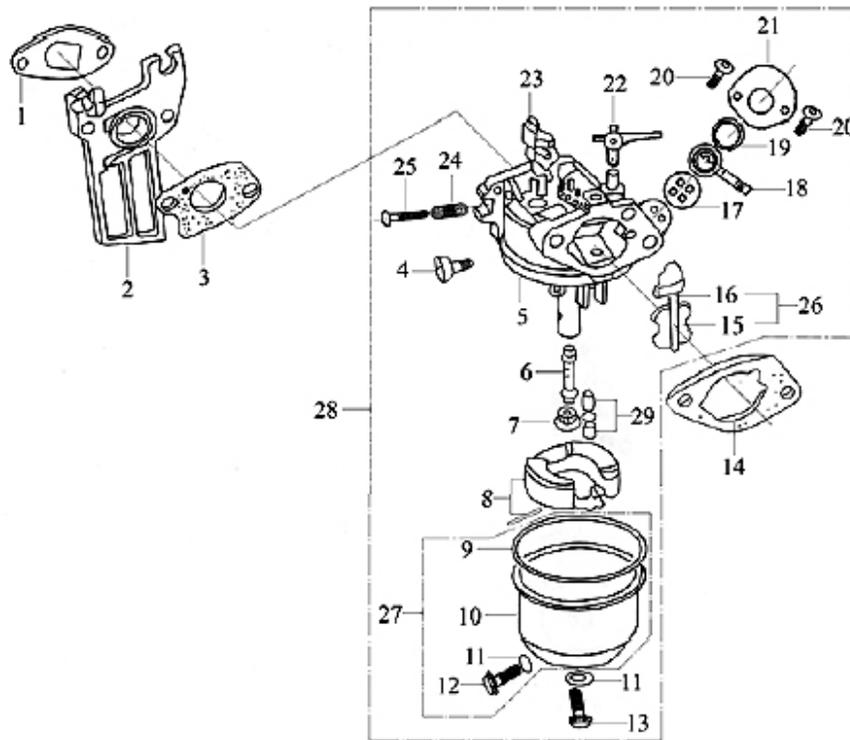
**Note:** When ordering parts from this list, specify: **Parts List F, CARBURETOR ASSEMBLY** and the ITEM No.
