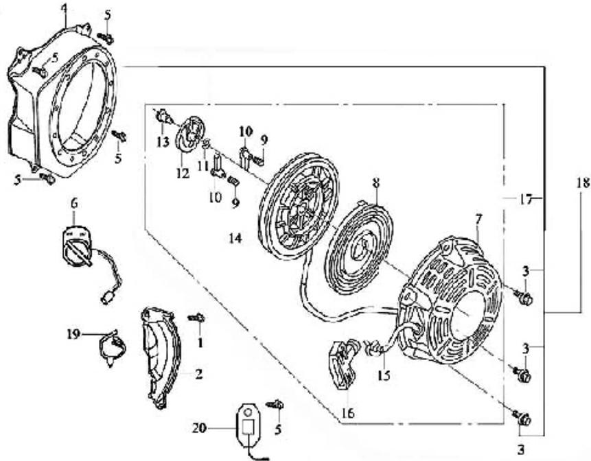
**Note:** When ordering parts from this list, specify: **Parts List K**, RECOIL STARTER ASSEMBLY and the ITEM No.
