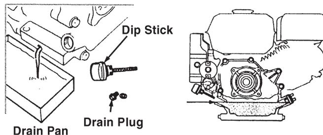
4. Allow all the oil to drain out into the pan. Pour the used oil into a container with a lid. Deliver used oil to a recycling center. Do not dump oil into the earth or storm drain. Dispose of oil properly.
