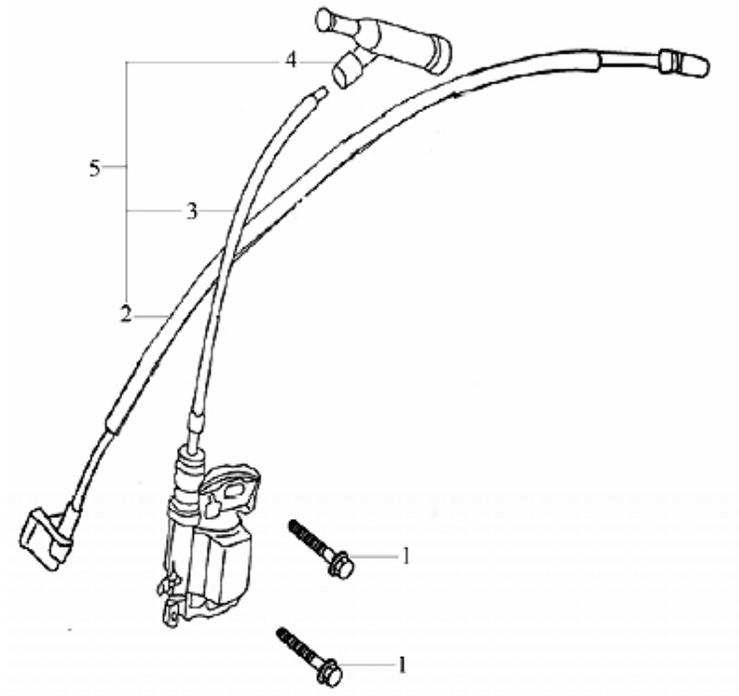
**Note:** When ordering parts from this list, specify: **Parts List N**, IGNITION COIL ASSEMBLY and the ITEM No.
