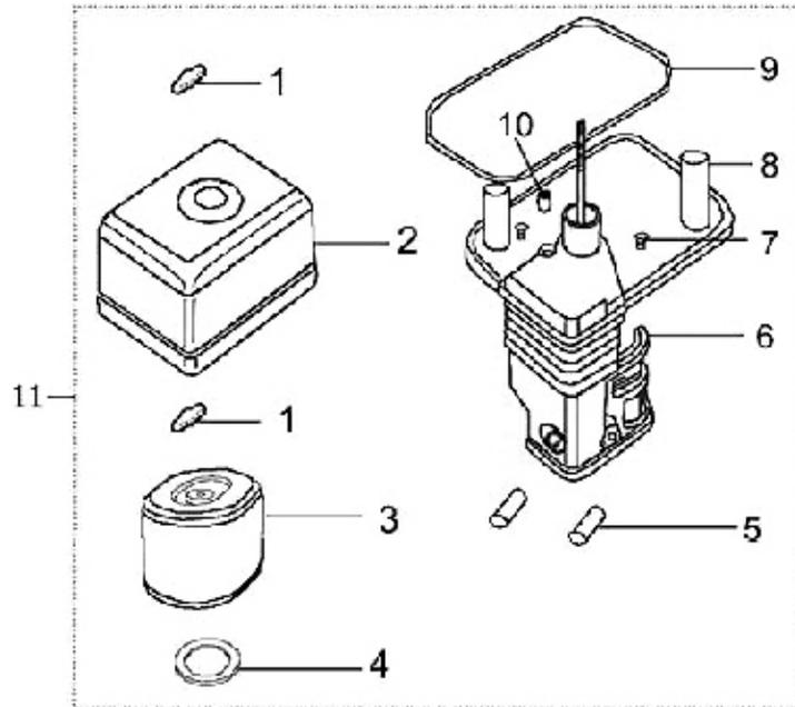
**Note:** When ordering parts from this list, specify: **Parts List H, AIR CLEANER ASSEMBLY** and the ITEM No.
