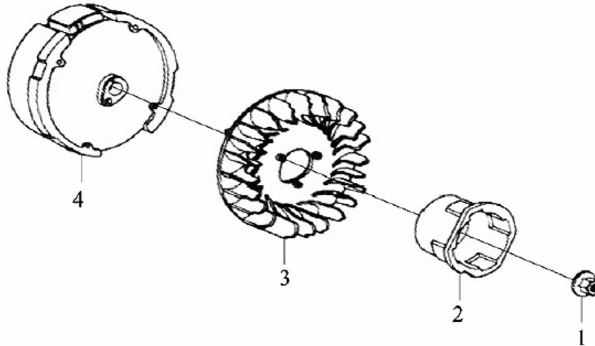
**Note:** When ordering parts from this list, specify: **Parts List M, FLYWHEEL ASSEMBLY** and the ITEM No.
