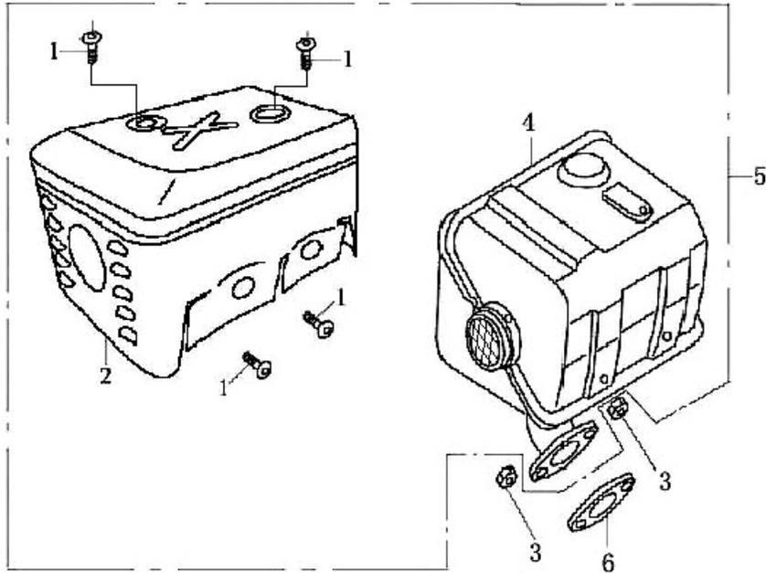
**Note:** When ordering parts from this list, specify: **Parts List J, MUFFLER ASSEMBLY** and the ITEM No.
