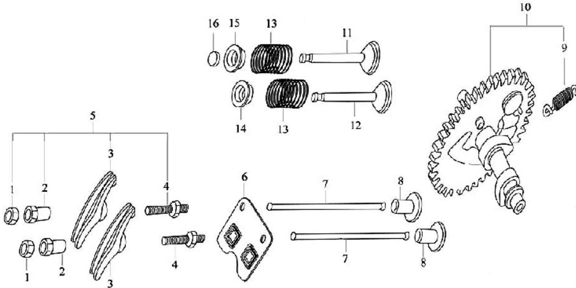
**Note:** When ordering parts from this list, specify: **Parts List E, CAMSHAFT AND ROCKER VALVE ASSEMBLY** and the ITEM No.
