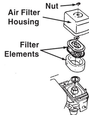
3. Check Air Filter. (See illustration above, right.) Unscrew Air Filter Wing Nut (1H) and remove the Air Filter Cover (2H) and Filter Elements. If dirty or dusty, clean (refer to the Maintenance Section).
