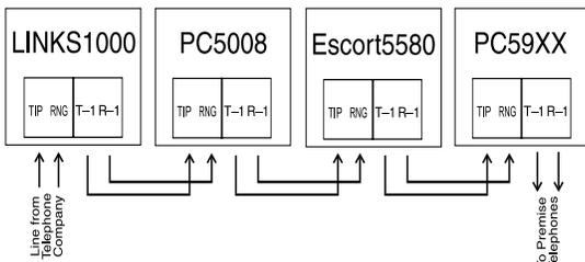
For example, if you are installing a PC1555MX with a LINKS1000 and a PC5928 Intercom module, connect the incoming line to the LINKS1000, then from the LINKS1000 to the PC1555MX, then from the PC1555MX to the PC5928 Intercom and then from the PC5928 to the house telephones.
