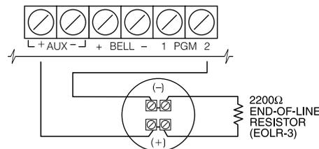
**NOTE:** If PGM2 is programmed for 2-wire smoke support, the connector JP1 on the main board must be removed.
