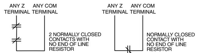
To enable normally closed loops, programming section [013], option [1] must be ON.
