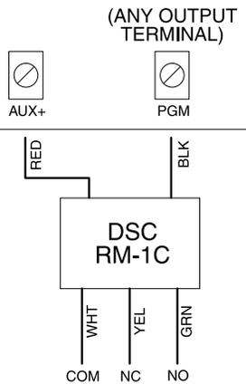
PGM1 can sink up to 50mA of current. Connect the positive side of the LED or buzzer to AUX+, the negative side to PGM1. PGM2 operates similarly to PGM1. However, PGM2 can sink up to 300mA of current. If more than 300mA of current are required, a relay must be used.
