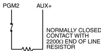
**NOTE:** If PGM2 is programmed for 24-Hr Auxiliary Input support, the connector JP1 on the main board must be removed.
