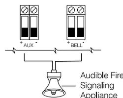
For UL installations, when a bell or siren is used for fire signaling with a pulsed cadence, it must be connected between the AUX+ and BELL- terminals. To maintain bell circuit supervision, do not connect more than one device to the BELL-terminal. A fire bell or siren used for
