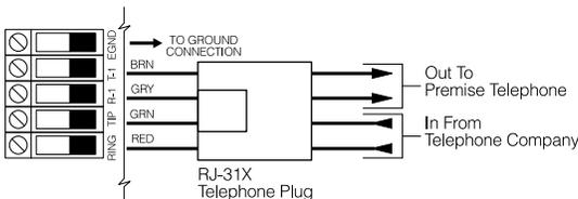
Connect the PC1555MX and modules which use the telephone line(s) in the following order:
