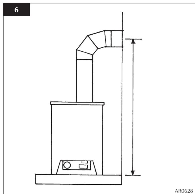
**TAKE CARE WHEN MARKING OUT FOR THE FLUE. IT IS DIFFICULT TO MOVE AFTER INSTALLATION.**
