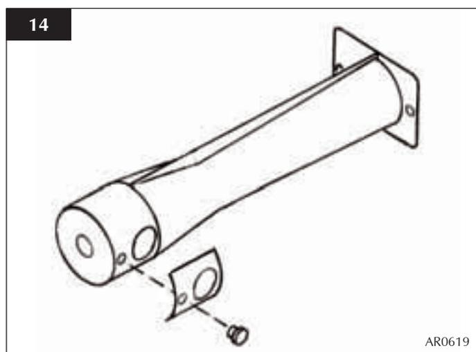
9.5 Reassemble in reverse order with correct aeration plate(s).
