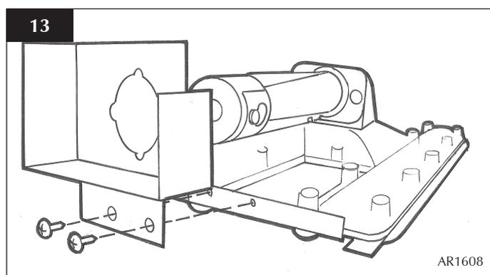
9.4 Refer to the technical specification and databadge to check the gas type and its required aeration plate. Change the aeration plate, if necessary.
