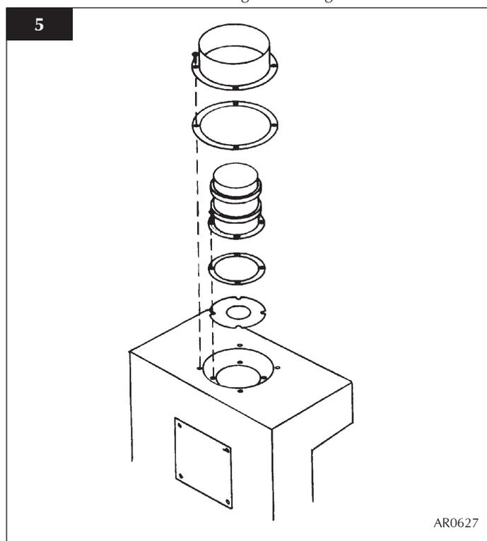
3.2.3 If the horizontal terminal is used assemble the required amount of vertical flue including the 90° elbow onto the stove. Drill through the fixing hole in the spigot using a 3.5mm drill and secure with the screw provided. Do not forget the optional decorative collar if you have purchased one. A wall plate is supplied to secure the flue to the inside wall. Bend the tab to 90° and loosely place on the elbow.
