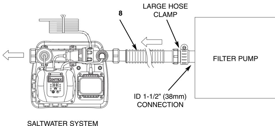
1. Connect the connector hose (8) to the filter pump outlet connection with a large hose clamp. Tighten securely.
