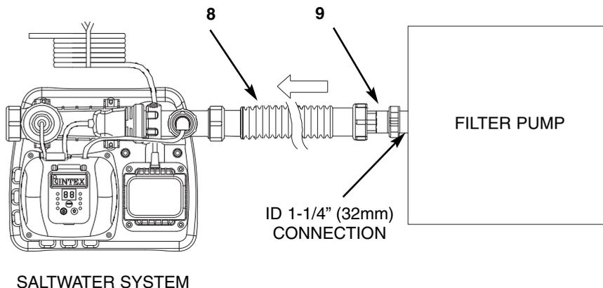
1. Connect one end of adaptor B (9) to the connector hose (8). Tighten securely.
