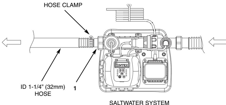
1. Connect the adaptor A (1) to the electrolytic cell (4) outlet. Tighten securely.
