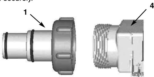
3. Disconnect the water return hose from the filter pump connection and connect it to the adaptor A (1) on the Saltwater System with a hose clamp. (see Drawing #1)
