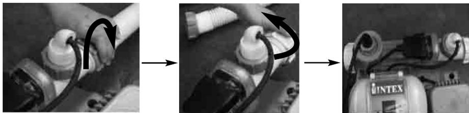
4. In a counter-clockwise motion, unscrew the collar of the copper electrode (5) and remove it from the electrolytic cell (4). Lift up the copper electrode.
