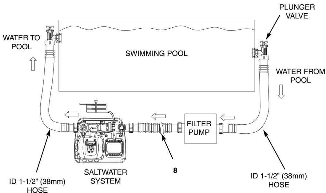
1. Go directly to step 2 if your pool is empty. If your above-ground-pool is filled with water, close the plunger valves before installing the Saltwater System.
