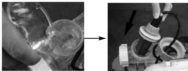
6. Open one side of the cell cover (10), drain and properly dispose of the vinegar. Connect the hose which goes from the pool to the cell. Flush the cell with the pool water.
