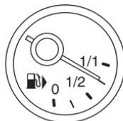
The symbol of the fuel pump with the arrow points to the side of the vehicle that the fuel filler inlet is located.
