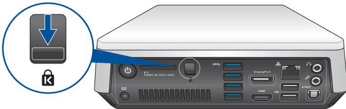
3. Slide the top cover towards the rear of the VivoPC until it is detached from the chassis.
