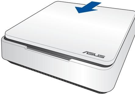
19. Lock the latch to securely fasten the top cover to the chassis.
