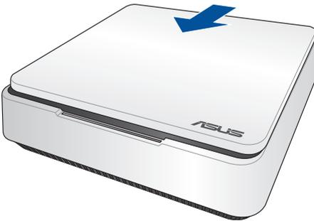
15. Lock the latch to securely fasten the top cover to the chassis.
