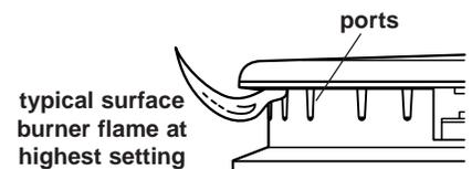
**D.** Check flame on “HI” for a blue color. It should be clean and soft in character. No yellow tip, blowing or lifting of flame should occur. Occasional orange flashes are normal and reflect different elements in the air or gas.
