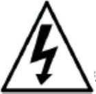
This symbol is intended to alert the user of the presence of uninsulated "dangerous voltage" within the product's enclosure that may be of sufficient magnitude to constitute a risk of electric shock to persons
