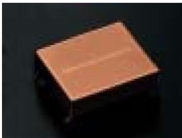
requirements of Marantz. Marantz developed its own discrete circuit boards to replace the IC's. These HDAM's consists of discrete surface mount components with short mirror image L/R signal paths. These devices are
