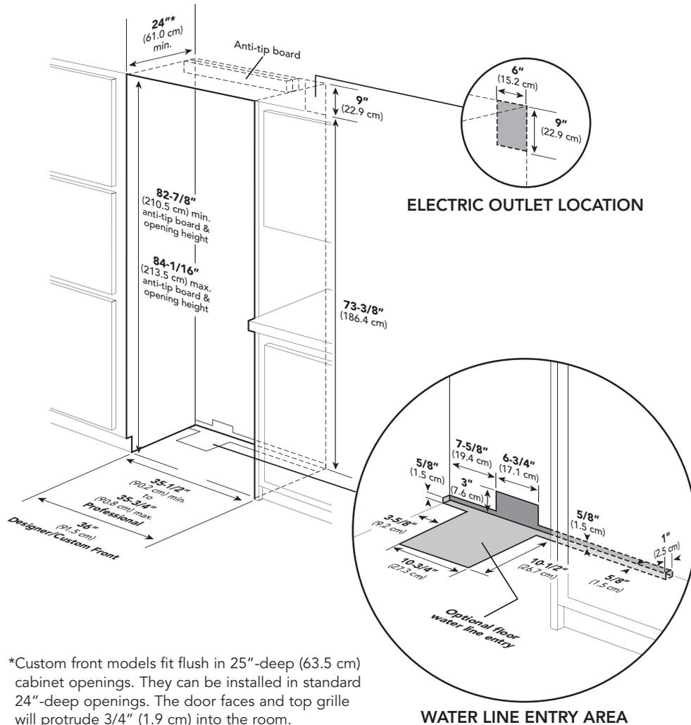
\*Custom front models fit flush in 25"-deep (63.5 cm) cabinet openings. They can be installed in standard 24"-deep openings. The door faces and top grille will protrude 3/4" (1.9 cm) into the room.
