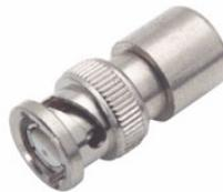
When pulling cables on STS systems, disconnect the cable at the splitter end first, and immediately install a terminator. Then, disconnect the cable at the STS card end. When reconnecting, connect the cable at the splitter end first. Then, remove the terminator at the splitter assembly and immediately connect the STS cable.
